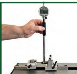
Setting 2-point bore gauges
